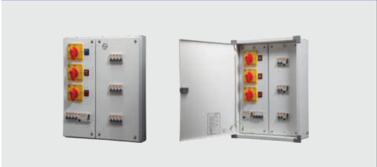
Metal DBs for Three Phase and Neutral (TPN ) supply distribution with selector switches for phase selection
